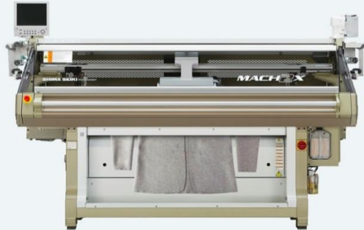
3D kötőgép (Ministry of Supply's '3D Print-Knit')
